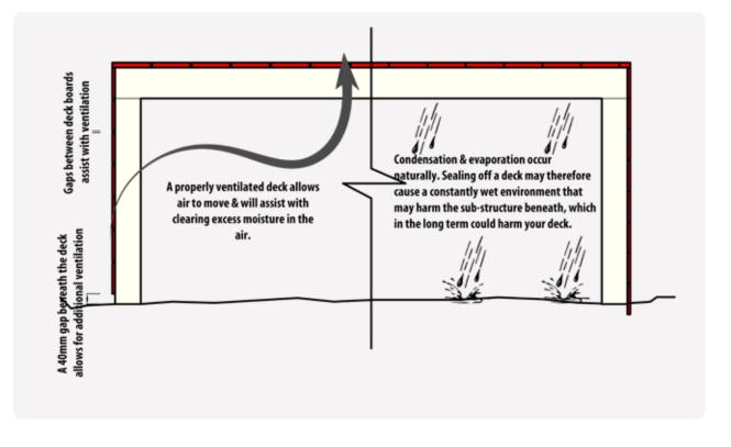
For non-screed surfaces, plan a minimum of 100 mm elevation space between the ground and the bottom of your lowest bearer. For screed surfaces, decking profiles must be elevated a minimum of 30 mm above the ground. This guideline is based on the smallest profile (composite batten) – other profiles may vary.
